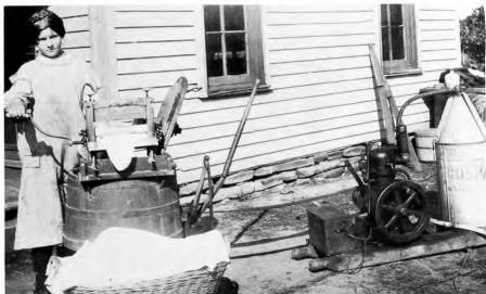
The approach of modern comforts — wash day lightened by a gas engine (about 1916).
